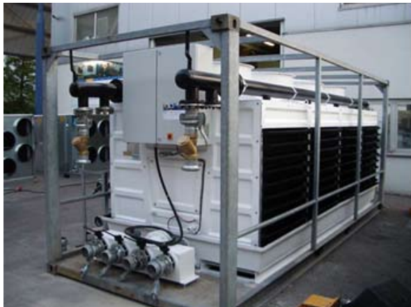
Cool Energy 2.5mW Rental Cooling Tower
